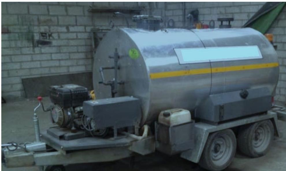
**Plate 3-7: Towable Sprayer for Temporary Reinstatement**
